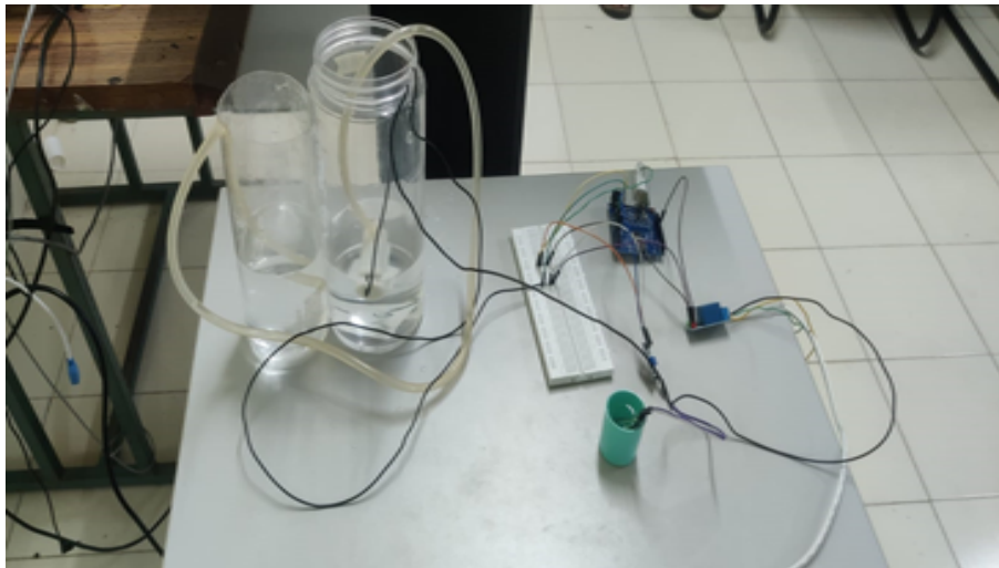
AUTOMATIC PLANT WATERING SYSTEM
